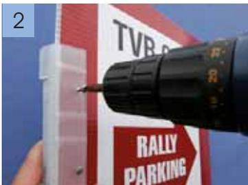
2 Secure the signAclip to the flute board by inserting 2 x 6 gauge screws into the clip.
