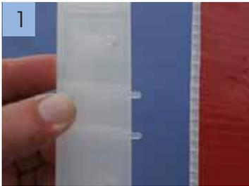
1 Insert the '4 x prongs' of the signAclip into the flutes of the flute board and push the clip all the way onto your sign.
