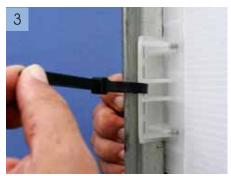
Slide the signAclip over a predrilled hole on the star picket, insert and tighten a single cable tie
